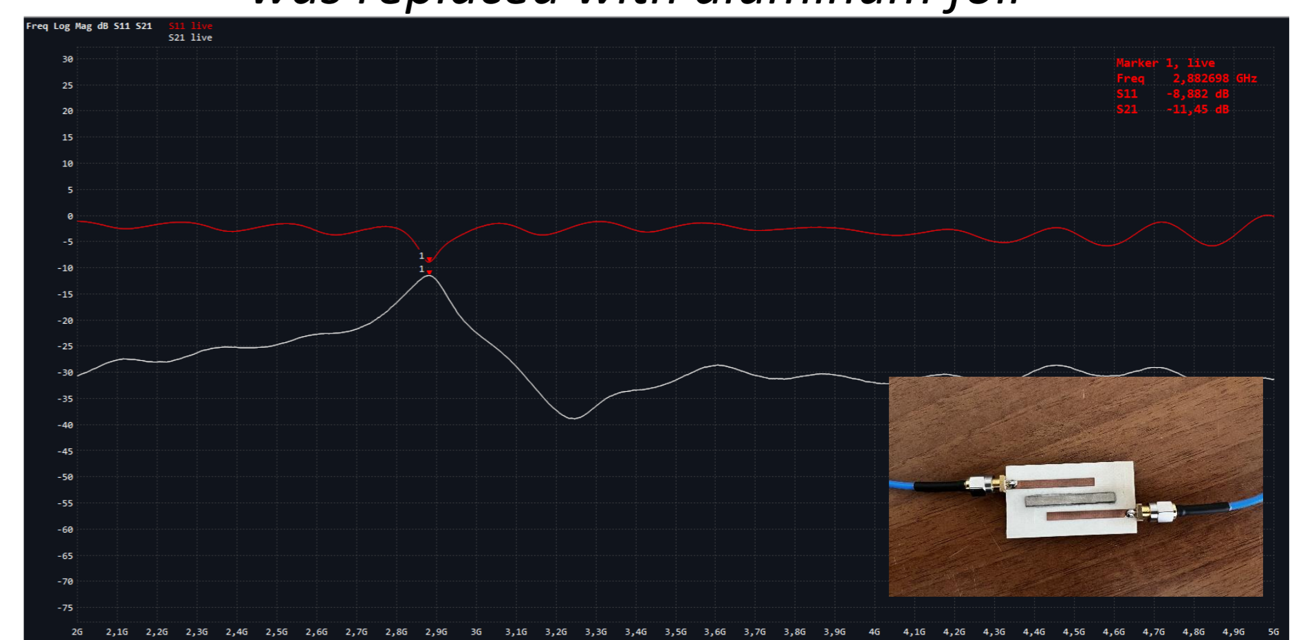
S-parameter results of the resonator that middle line was replaced with conductive textile
