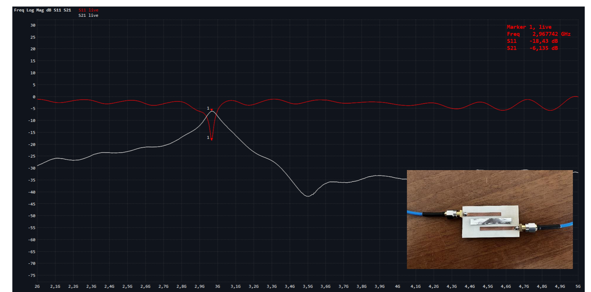
S-parameter results of the resonator that middle line was replaced with aluminum foil
